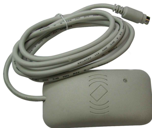
Figure 2: The external Equitrac smart card reader which is attached to every FollowYou printer
